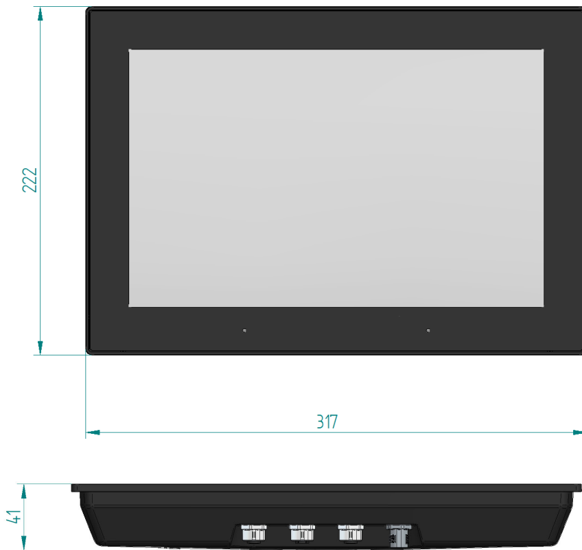
Figure 12: CCpilot V1200 dimensions
